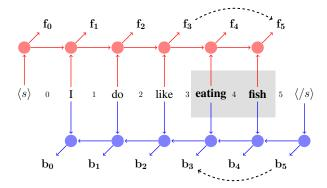
**Figure 3:** Word spans are modeled by differences in LSTM output. Here the span  $_3$  *eating fish*  $_5$  is represented by the vector differences ( $\mathbf{f_5} - \mathbf{f_3}$ ) and ( $\mathbf{b_3} - \mathbf{b_5}$ ). The forward difference corresponds to LSTM-Minus (Wang and Chang, 2016).
